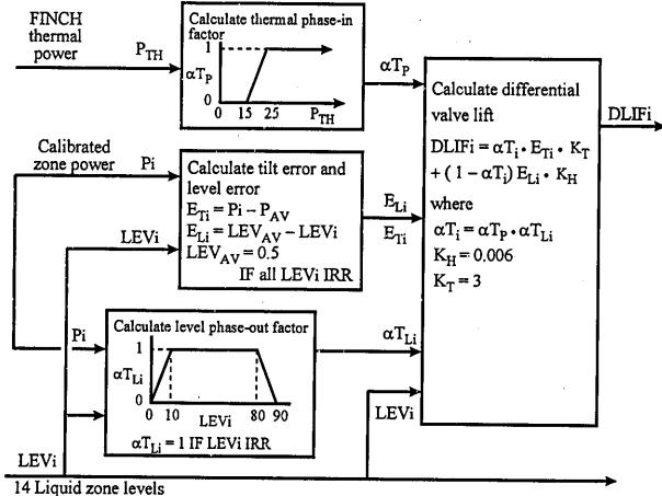
the zone power tilt error is the difference between the measured power in the given zone and the average of all the 14 zones; if the in-core detector readings are IRR then zone thermal power is used instead of the flux measurement
