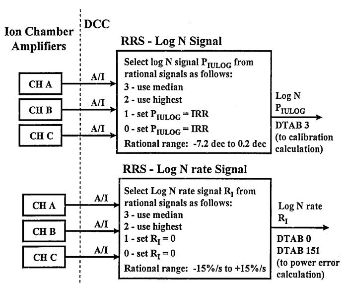
• output is R<sub>I</sub>, which is the actual Log N rate measurement. It is stored in RRS under the label DTAB 0 in units of decades/sec, and under DTAB 151 in units of %/sec.
